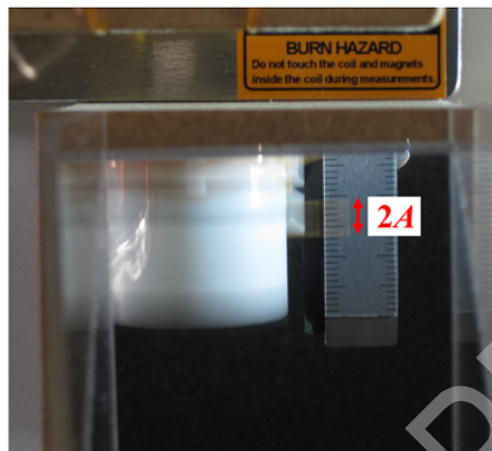
Figure 6: Oscillation behavior as seen through the mirror.
