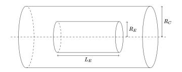
The emitter is heated so that there are always excess electrons available to be accelerated through the potential difference toward the collector. The electrons fill the vacuum with a plasma. Because of the properties of a plasma there is a maximum current that can flow through the diode that depends on the potential of the collector and the geometry of the system.
